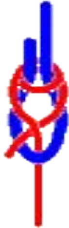
SHEET BEND Join 2 lines of unequal thickness
