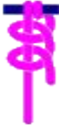
ROUND TURN TWO HALF HITCHES Line to post or ring
